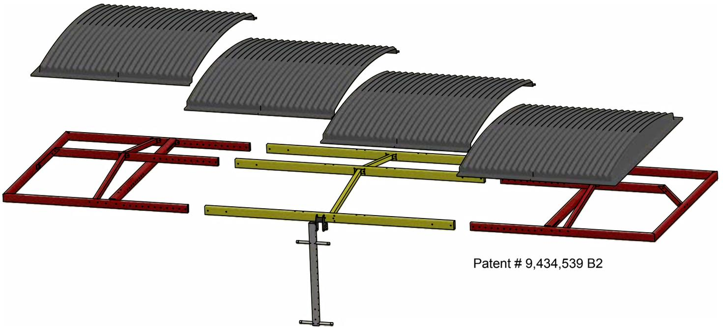
To ensure proper opening and closing functionality there will be a gap of up to 1" between the cover and top of container.
