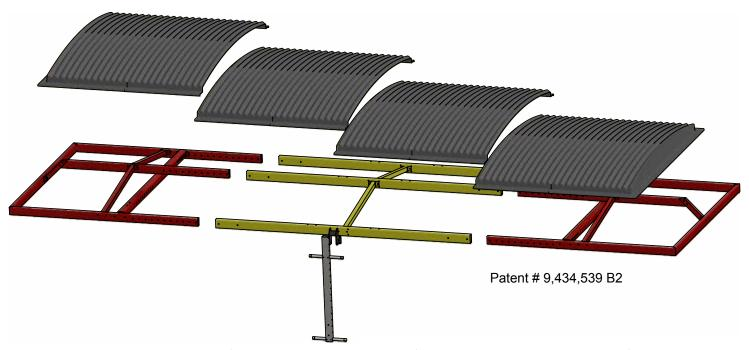
To ensure proper opening and closing functionality there will be a gap of up to 1" between the cover and top of container.
