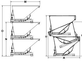
NOTE: The LH-50 and LH-100 stack. The LH-150, LH-200 and LH-250 nest.
